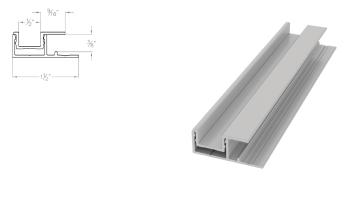
Note: Adhesive must be applied within the EZ.Lock™ Engagement Channel.
