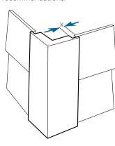
Fasten both sides according to standard AZEK Trim Guidelines. 4" Cornerboards may be installed using 2 fasteners at ends and splices and 1 fastener 12" OC through length of board.
