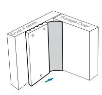
Firmly push Thermostop against Garage Door and fasten. Rubber seal should be in contact with Garage Door, but not overly tight. Place 2 fasteners within 1/2" of all ends and splices. All other fasteners should be 8" on center entire length of board.
