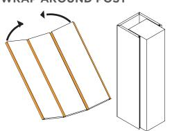
SNAP THE LOCKING **PANEL TO THE** THREE PANEL **COLUMN WRAP**
