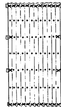
Fig. 10 CAUTION: Be sure to center endlaps on purlins and center nails on endlaps.
