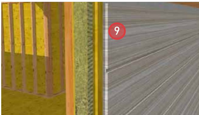
9. Install cladding. Provide venting at the top of the wall to allow for the free movement of air through the wall cavity. It is not recommended to vent the wall cavity into the roof.
