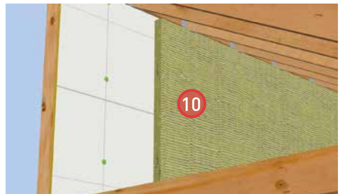
10. Install ROXUL® COMFORTBOARD™ 80 on the exterior of the wall between canopy ledger boards with recommended fasteners.
