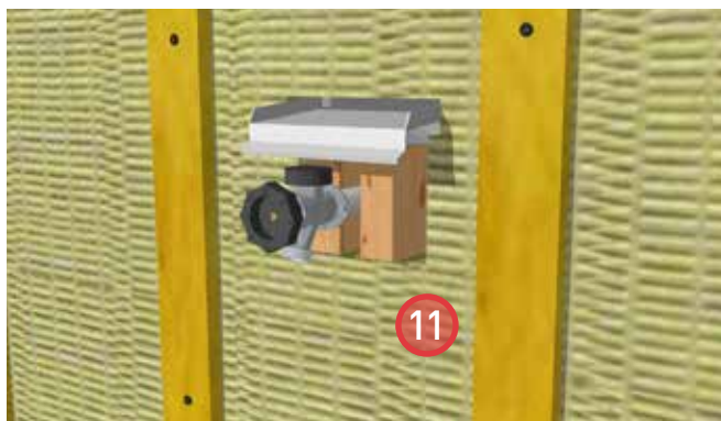
11. Install ROXUL® COMFORTBOARD™ 80 and strapping. Provide bugscreens at the top and bottom of the strapping.
