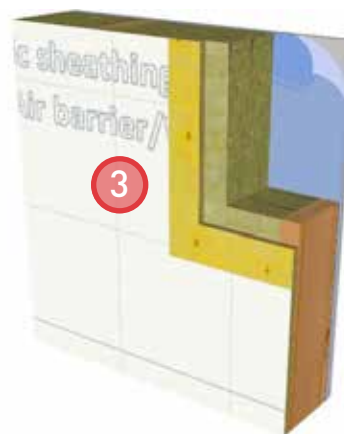
3. Install sheathing membrane.
