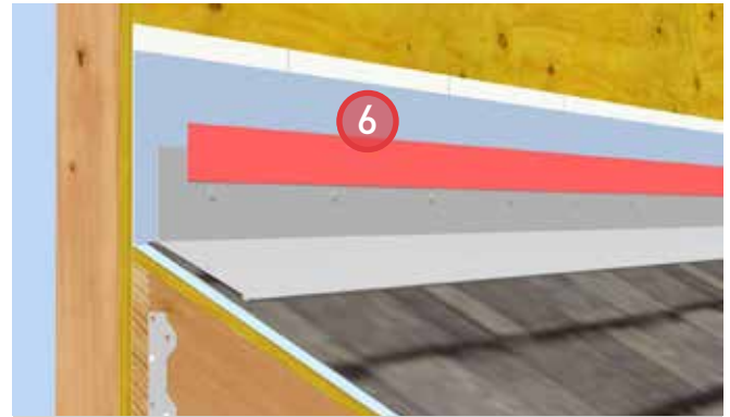
6. Install prefinished metal closure flashing and seal the leading edge with sheathing tape to provide for air barrier continuity.
