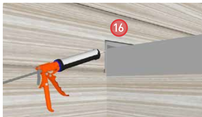
16. Install backer rod and sealant at the gap between the flashing and the cladding.
