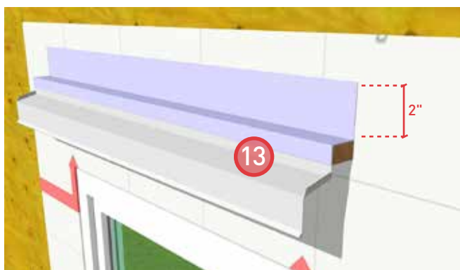
13. Install self-adhesive membrane over the prefinished metal flashing and extend 2" up the face of the wall.
