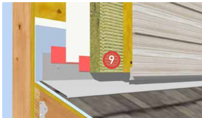
9. Install cladding and closure flashing.
