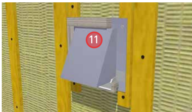
11. Install cladding and trim boards around the exhaust vent hood.
