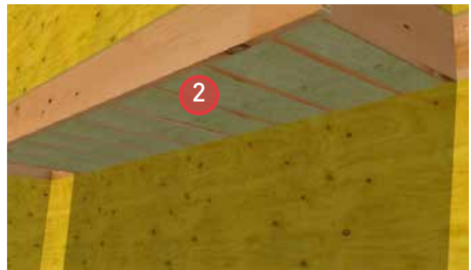
2. Install ROXUL® COMFORTBATT® in the cantilevered floor joist cavities. Ensure insulation extends through to the interior plane of the wall assembly to maintain thermal continuity.
