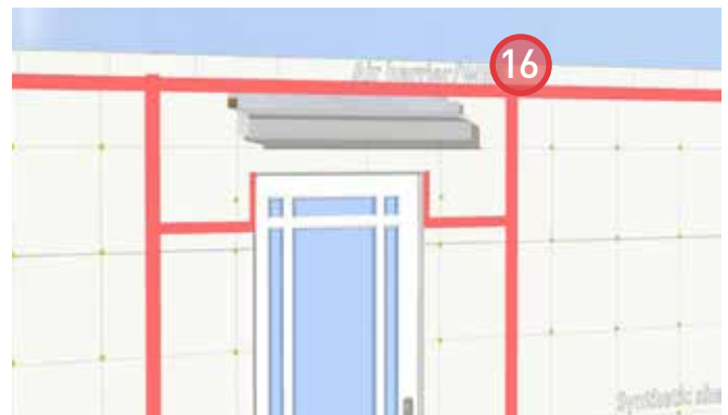
16. Install sheathing membrane from above and seal the leading edge with sheathing tape to maintain air barrier continuity. Ensure the sheathing membrane laps over membrane layers below.
