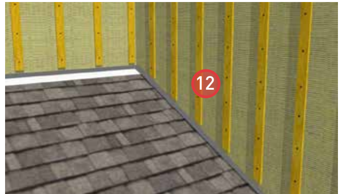
12. Install ROXUL® COMFORTBOARD™ 80 and secure in place with strapping. Provide bugscreens at the top and bottom of the strapping.
