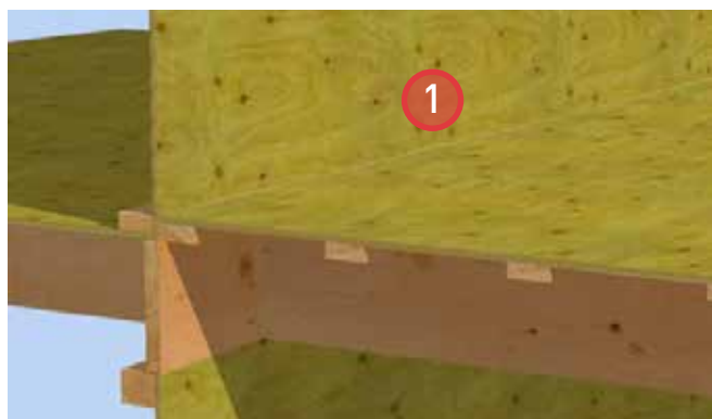
1. Typical wood frame construction at cantilevered balcony to above grade wall interface.
