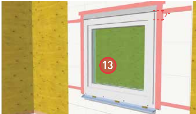
13. Install metal flashing at the head of the window. Seal the leading edge of the flashing with sheathing tape.
