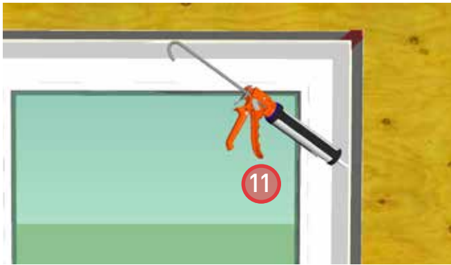
11. Install backer rod and sealant around the interior perimeter of the window to complete air barrier continuity.
