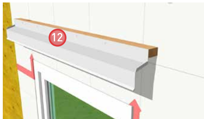
12. Install head flashing using wood blocks to space it beyond the insulation layer.
