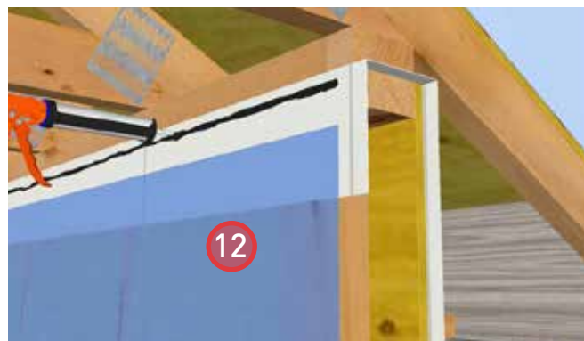
12. Install a bead of acoustical sealant to the sheathing membrane at the lower top plate to transition the air barrier from the wall to the ceiling.
