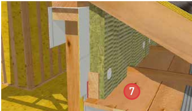
7. Install soffit materials and venting.
