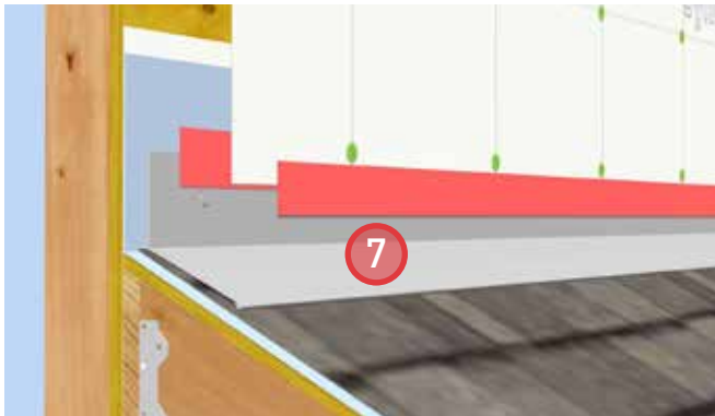
7. Install sheathing membrane. Lap the membrane over the closure flashing and seal the leading edge with sheathing tape to maintain air barrier continuity.
