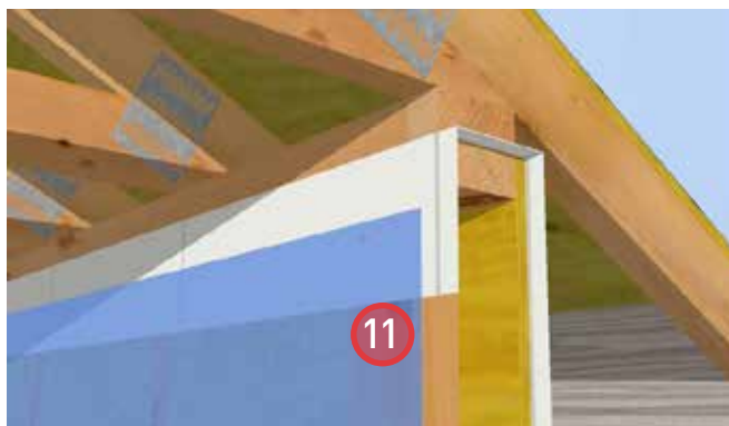
11. Install poly and fasten to the sheathing membrane at each stud with staples.
