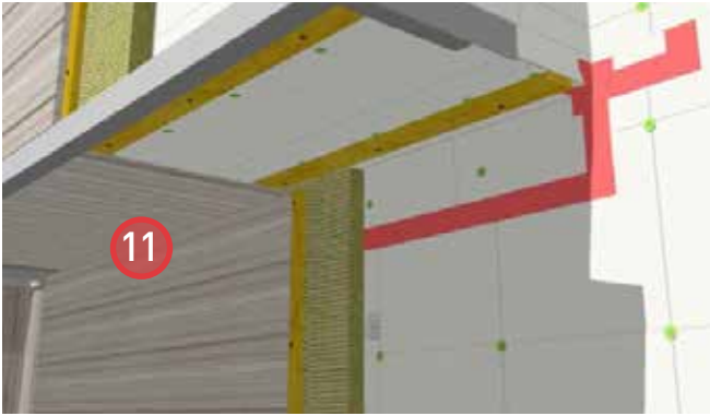
11. Install cladding and vented soffit material.
