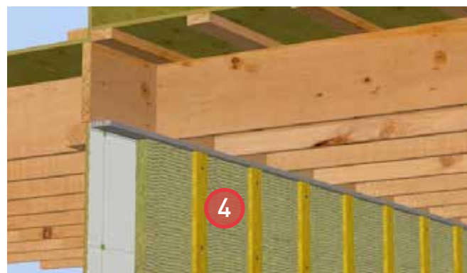
4. Install ROXUL® COMFORTBOARD™ 80 and strapping with bugscreens, leaving a \frac{3}{4} " gap between the insulation and the top of the wall. Suggest using a 1x4 temporary spacer board to space the insulation.
