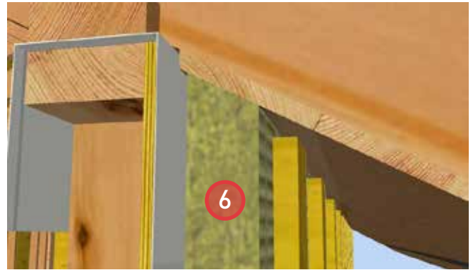
6. Install ROXUL® COMFORTBOARD™ 80 and strapping to the exterior of the wall. Provide bugscreens at the top and bottom of the strapping.
