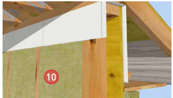
10. Install ROXUL® COMFORTBATT® within the interior stud cavities.
