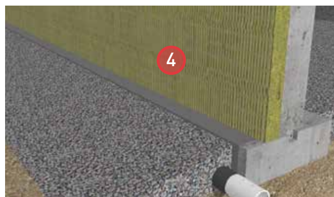
4. Install ROXUL® rigid board insulation against foundation wall. Spot adhere the insulation to prevent puncture of the waterproofing membrane.
