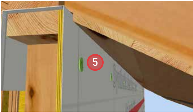
5. Install soffit material and vents.
