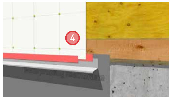
4. Install sheathing membrane and seal leading edge to the flashing with sheathing tape to complete air barrier continuity. Provide a \frac{3}{4} " vision line on the flashing backleg.
