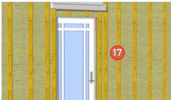
17. Install ROXUL® COMFORTBOARD™ 80 and secure in place with strapping. Provide bugscreens at the bottom and top of the strapping.
