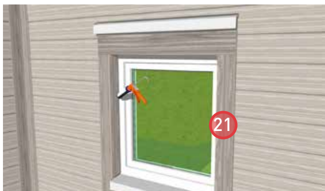
21. Install sealant around the perimeter of the window between the trim boards and the window frame (top and sides).
