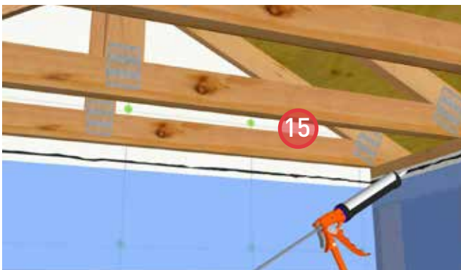
15. Install a bead of acoustical sealant along the sheathing membrane in line with the lower top plate of the exterior wall.
