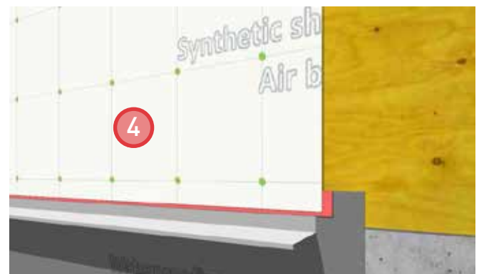
4. Install sheathing membrane and seal leading edge with sheathing tape to complete air barrier continuity. Provide a \frac{3}{4} " vision line on the flashing backleg.
