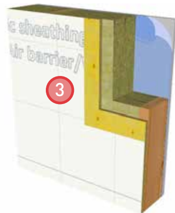
3. Install sheathing membrane.
