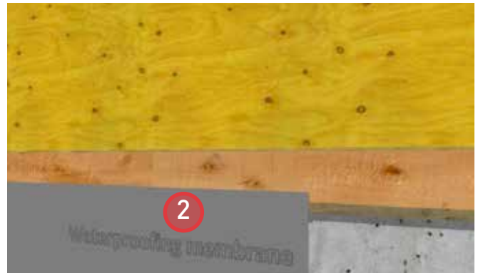
2. Install below-grade waterproofing membrane. Provide a 2" overlap of waterproofing membrane onto the sheathing.
